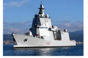
Class: Multipurpose Offshore Patrol Boats (PPA) Commissioned: 2017 Displacement: 6679 tons Lenght: 143 m Beam: 16.5 m Engine system: Code Speed: 32 Kts (Max)
