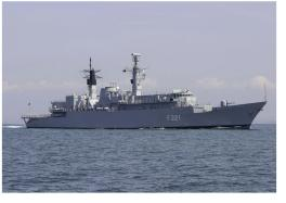
Max displacement: 4800 tons fully loaded Total lenght: 148 meters Beam: 14,7 meters Draft: 6,4 meters Speed: 30 kts (Max)/18 kts (Cruise)/14 kts (Eco) Powerplant: 2 Olympus turbines and 2 ST40M turbines
