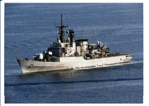
Displacement: 3040 tons fully loaded Lenght: 123 m Beam: 12,9 m Draft: 6,3 meters Speed: 30 kts Powerplant: 2 Gas Turbines Fiat-General Electric LM-2500 and 2 Diesel engines Warstila B230-20 MVM (50000 KW); 4 Diesel Generators (975 kW each); 2 shafts with variable pitch propellers
