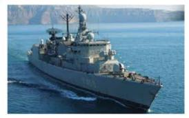
Displacement: 3630 tons Lenght: 130 meters Beam: 14,6 meters Draught: 6,2 meters Maximun Speed: 32 knots Propulsion: 2 RR Olympus TM3B 56.800 HR, 2RR Tyne 10
