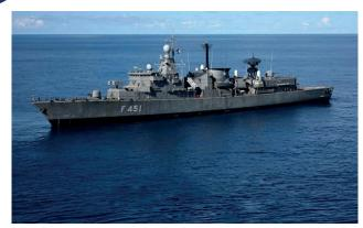
Displacement: 3500 tons Length: 130 meters Beam: 14,6 meters Draught: 6.2 meters Maximum Speed: 30 knots **Propulsion**: 2 Gas Turbine Rolls Royce Tyne RM1C 2 Gas Turbine Rolls Royce TM3B
