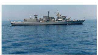
Displacement: 3500 tons Length: 130 meters Beam: 14,5 meters Draught: 4,4 meters Maximum Speed: 30 knots Propulsion: 2 Gas Turbine Rolls Royce Tyne RM1C 2 Gas Turbine Rolls Royce TM3B
